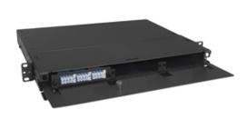
OptoSpan Part# HPP9-LDZLDZ-1XF is a Matrix-HD Series high density, modular (LGX Fiber Adapter Panel), fullyloaded Single-mode LC Flat 1U fiber patch panel. It is a complete LGX Fiber Adapter Panel based turnkey solution with a total of24 LC fibers (12 Duplex LC) in 1U. This modular fiber patch panel is factory pre-loaded with Qty. 1 24 fiber LC Duplex LGX Fiber Adapter Panels for quick implementations in 10/100G networks.
