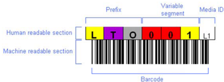
Figure 1. Parts of the LTO label
