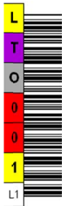
Figure 4. Right barcode orientation
